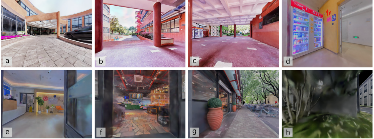
Figure 4: Representative L1 failures. Exit: (a) timeout without STOP after reaching outdoors; (b) premature STOP before crossing outside. OVON: (c,d) failure to recognize a visible vending-machine goal. Entrance: (e,f) premature STOP outside a doorway; (g) timeout without entering a visible entrance. OutdoorNav: (h) repeated forward motion into vegetation, resulting in stagnation.
