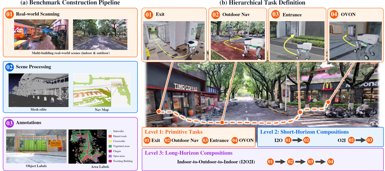
Figure 2: Overview of I2O2I-Nav. (a) Benchmark construction pipeline. Large-scale real-world indoor–outdoor environments are scanned and processed into executable navigation scenes with collision geometry and navigation maps, together with object-level and area-level semantic annotations. (b) Hierarchical task definition with increasing compositional complexity. Level 1 evaluates four primitive tasks: Exit, Outdoor Navigation, Entrance, and Open-Vocabulary Object Navigation (OVON). Level 2 evaluates two-stage compositions, Indoor-to-Outdoor (I2O) and Outdoor-to-Indoor (O2I), where the second stage continues from the state reached by the first. Level 3 composes all four primitives into a continuous long-horizon I2O2I mission.
